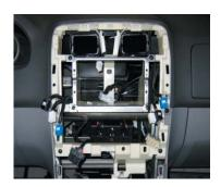
Place the head unit including mounting plates and supporting bracket.
