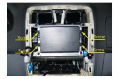
Remove 4 screws and remove the panel.
