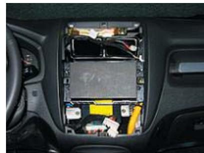
Use a plastic wedge to remove the panel and remove 4 screws.
