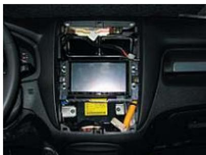
Place the headunit including mounting plates and supporting bracket.
