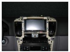
Place head unit including mounting plates and supporting bracket.
