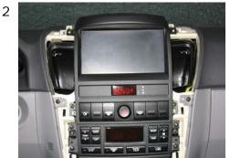
Use plastic wedge to remove panel on left and right side.
