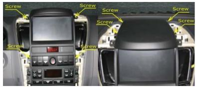
Remove 8 screws and remove front en upper panel complete.
