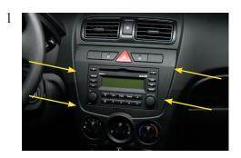
Remove the dashboard panel at the location of the arrows. By using a plastic wedge.
