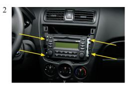
Remove the original radio. This is thighten by four screws.
