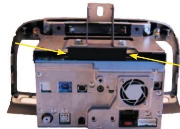
Place the mounting block on the rear of the new headunit between the metal bracket and the new headunit.
