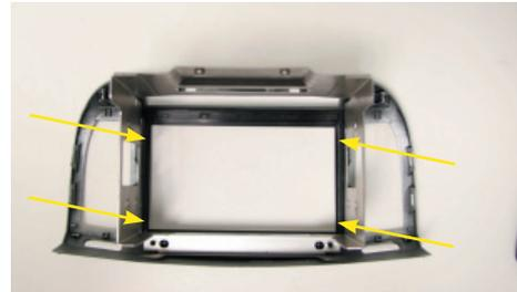
Remove the original headunit from the dashboard panel. Place the replacement panel behind the dashboard panel.
