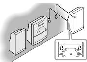
• The heat radiation from the rear of the main unit may deform or discolor the wall made of certain material.
