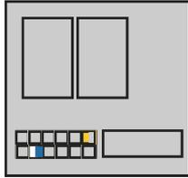
The command wires are on the FAKRA connector at position 6 and 8.
