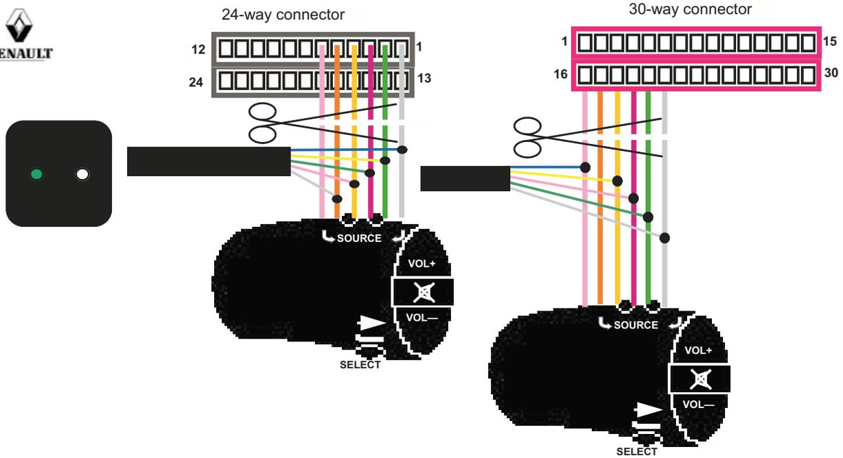
For the 30-way connector, cut the wires from position 16 until 22. For the 24-way connector, cut the wires from position 1 until 6. Connect the CAW-COMUN1 wires towards the steering wheel side. Once finished the connections, connect the OEM connector in it's place on the display
