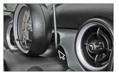
7. Remove 2 screws of the rev counter
