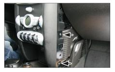
10. Unclip and remove side panels of the center console Remove 4 screws(2 at each side)
