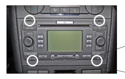
. Insert four Ford Mondeo radio release keys in the OEM head unit.
