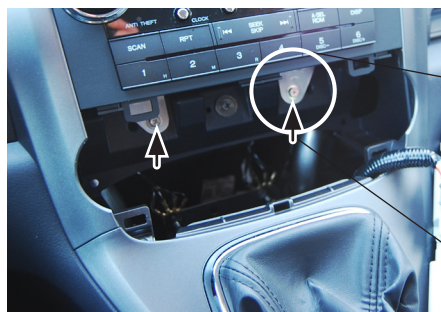
3. Remove the two screws below the OEM head unit
