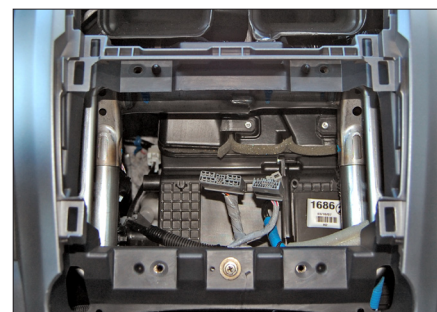
6. Remove the OEM head unit
