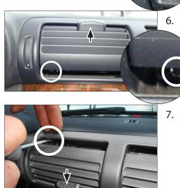
Unclip the air vent unit carefully on both sides with a screw driver.
