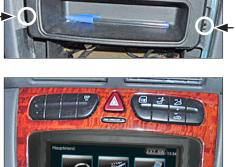
Remove the four Torx screws (2 on each side) holding the OEM head unit.
