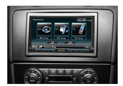
3. Place the facia plate on the dashboard. Fix it with the 2 original screws.
