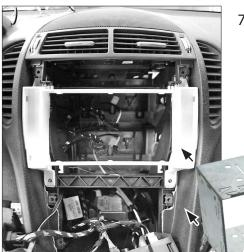
Place the mounting frame at the dashboard. Fix it with the original screws.
