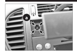
Open the cup holder above the OEM head unit. Remove screws (a) and (b). (The screws are covered with rubber caps)
