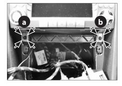
Remove screws (a) and (b) Remove OEM head unit.
