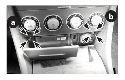
Open the ash tray Remove screw (a) on the left. Remove the cover surrounding the cigarette lighter. Remove screw (b) on the right.
