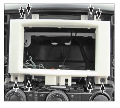
3. Dashboard with removed OEM radio and aircon control unit.
