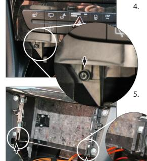
4. Remove the control unit / or CD-Changer underneath the OEM radio by removing the screws at left and right side
