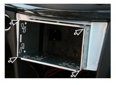
7. Push the metal frame into the mounting bracket
