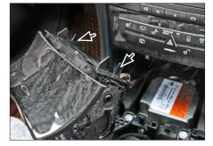
Open the ash tray and remove the complete ash tray unit
