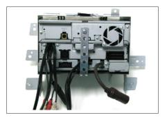
6. Tighten the headunit onto the metal band. Various positions are possible.
