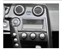
7. Place the metal bracket including the headunit. Connect all required wires.
