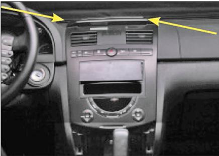
2. Remove the speaker grill on top of the dashboard. Remove the two which have become visible.
