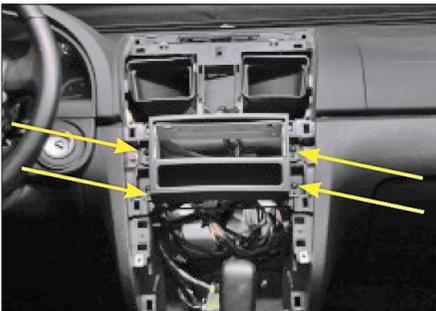
3. Remove the original bracket. This is tighten by screws.
