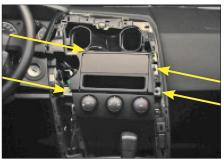
Remove the original bracket, which is tighten by four screws at the location of the arrows.
