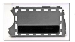
Remove the original plastic bracket from the metal bracket, which is tighten by four screws.
