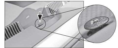
4. Open up the top glove box cover, remove the plastic screw located on the inside, gently.
