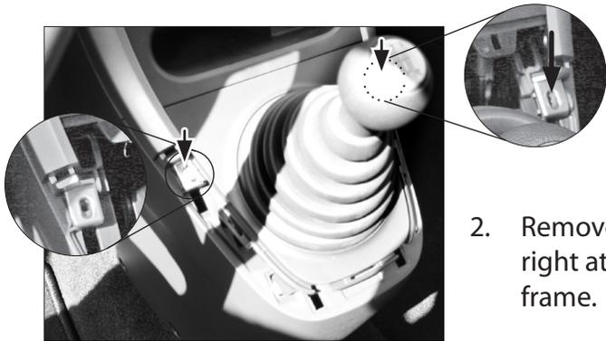
2. Remove the 2 screws left and right at the base of the silver trim frame.
