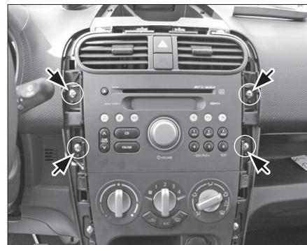
6. Remove the 4 Phillips screws, remove the OEM Radio.
