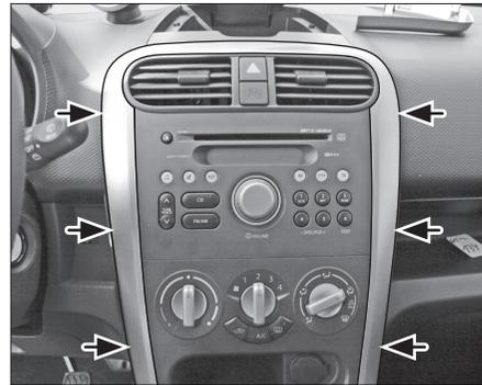
5. Remove the thin silver trim frame, which is clipped to the dashboard.
