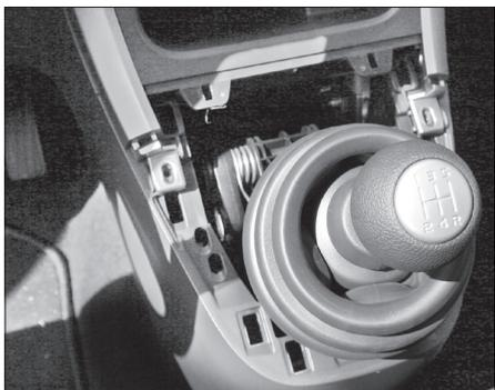
3. Remove the gear lever cap.
