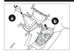
1. Remove the shift knob (a) and shift cover panel (b).
