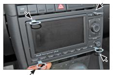
2. Use 4 radio release keys to dismount the OEM radio.
