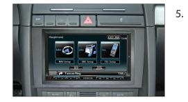
Connect alle required circuit points and push the double DIN head unit until it snaps in.
