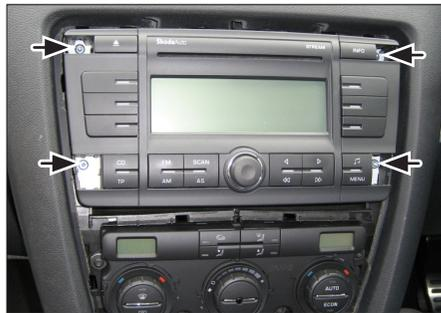
2. Remove 4 screws fixing the OEM head unit. Remove OEM head unit.
