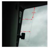
• \*/ Where the earth sheet of the Amplifier (a) can be stuck on the metal part of the front pillar.
