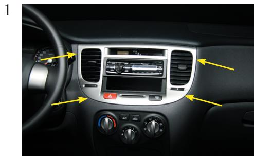
Remove the panel around the original radio.
