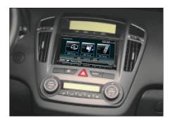
Connect all required circuit points to the Pioneer head unit and push it into the metal frame until it snaps in. Place the facia plate.
