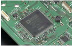
For main IF DSP, transmission unit ADSP-21363 clock @333 MHz
