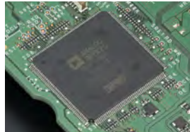
For sub IF DSP, every kind of signal processing ADSP-21369 clock @260 MHz
