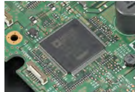
For band scope ADSP-21363 clock @333 MHz
