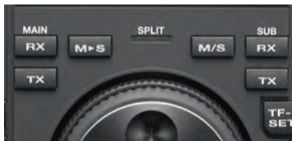
Fig. 101 Key Allocation Suitable for Split Operation
