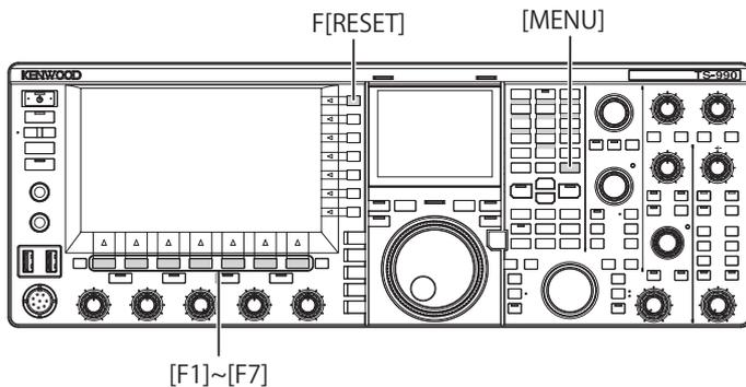
Follow the procedure below to reset the transceiver.
