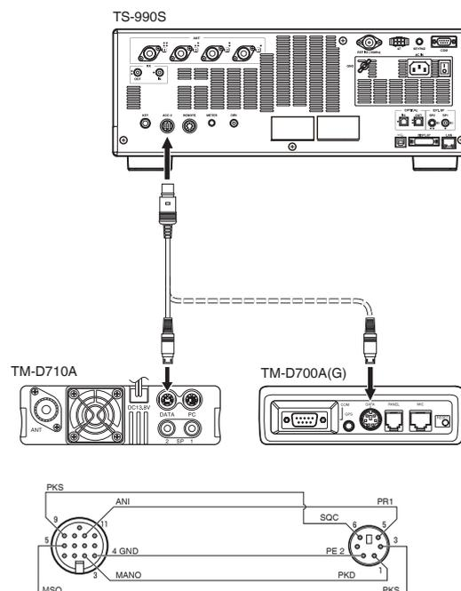
Be sure that "On" has been configured for both Advanced Menus 14, "PKS Polarity Reverse", and 15, "TX Inhibit While Busy". Refer to "INHIBITING THE TRANSMISSION DURING BUSY (SQUELCH OPENING)" and "REVERSING THE PKS SIGNAL POLARITY" for the configuration methods.
