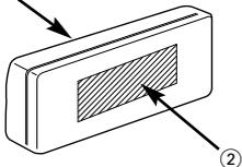
Attach one strip of Velcro to the slanted-line of the display units as shown to the left, and attach the other strip of Velcro to the parts where you wish to attach the display units. Then, put velcros together and install the display units.
