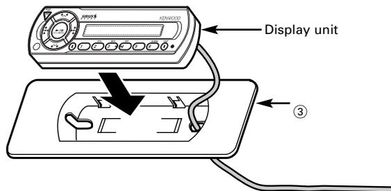
Pass the wire from the display unit through the hole on the trim mount plate and push fit the display unit into the trim mount plate until it locks.
