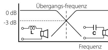
$$L = \frac{159 \times R}{f_c} \text{ (mH)} \quad C = \frac{159000}{f_c \times R} \text{ (\mu F)}$$
