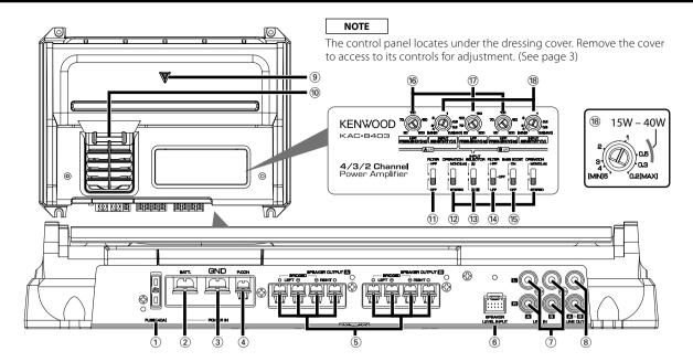
This is a 4 channel amplifier including 2 stereo amplifiers in a body. One amplifier is referred to as amplifier A and the other is amplifier B. This unit is compatible with a large variety of systems by combining the switches and functions described in the following.
